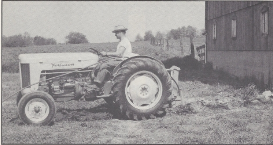
Fig. 5 Laying Plastic Pipe with the Tube and Cable Laying Attachment
